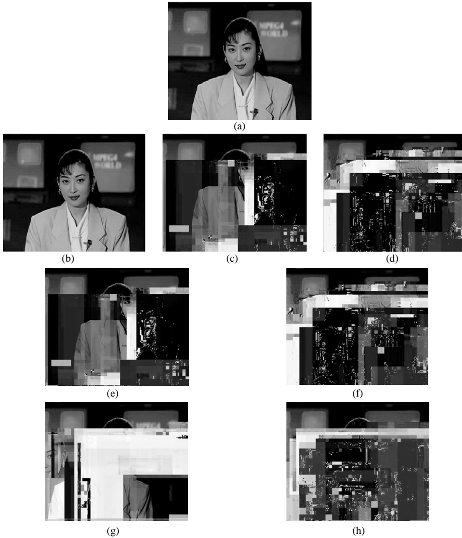
Fig. 11. (a) MPEG-4 encoded original sequence; Decoded video after simulated transmission using traditional 802.11b protocol stack at (b) 2 Mbps, (c) 5.5 Mbps and (d) 11 Mbps; using UDP (with MAC Lite) at (e) 5.5 Mbps and (f) 11 Mbps; using UDP Lite (with MAC Lite) at (g) 5.5 Mbps, (h) 11 Mbps.
