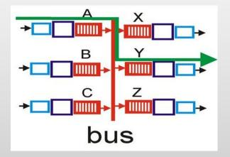
1 Gbps bus in Cisco 1900: sufficient speed for access and small enterprise networks (not ISPs)
